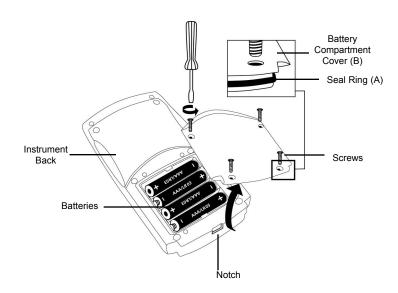
To ensure that the instrument is waterproof:
